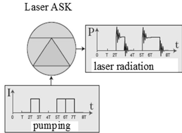
Fig. 2. Modulated laser radiation with direct modulation.
