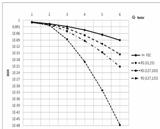
Fig. 5. BER as a dependency from a communication line power budget with different RS code types.
