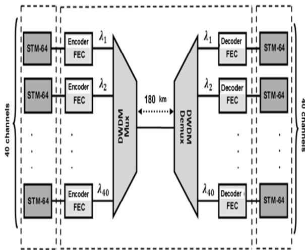
Fig.3. The simplified diagram of DWDM systems.
