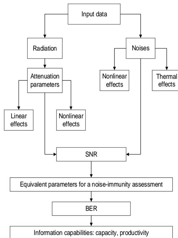
Fig.1. The calculation methodology of the FOCL information capabilities
