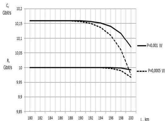
Fig. 6. The data transmission and productivity as a function of the fiber-optics line length.
