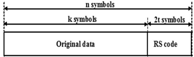
Fig. 4. The data block on the RS encoder  $(n, k)$ .
