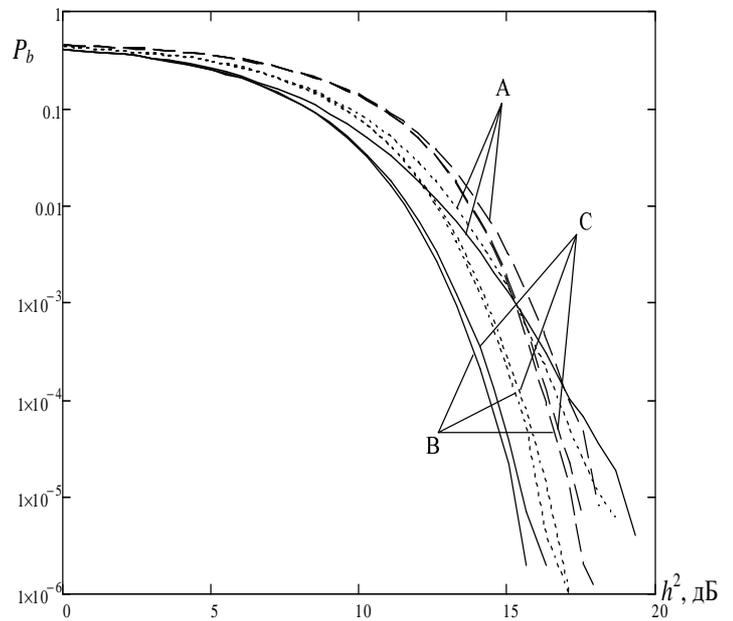
Fig. 12. The dependence of the bit error probability  $P_b$  versus the signal-to-noise ratio  $h^2$ : A — Gaussian distribution of useful signal; B — the binary distribution, C — symmetrized beta distribution
