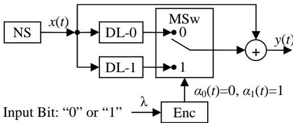
Fig. 4. CDNSK transmitter block diagram
