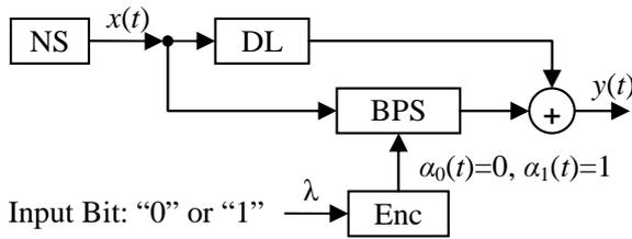
Fig. 7. Block diagram of Voronin system transmitter
